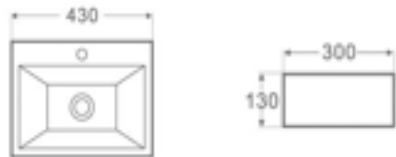
235 Art Basin Size: 430x300x130mm Wall mounted-supplied with screws
